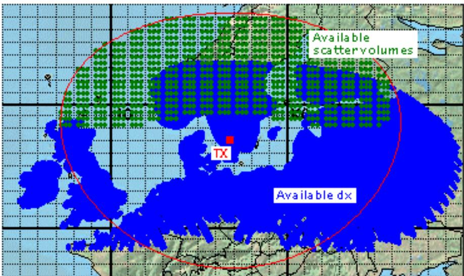
**Figure 3.** Available scatter volumes (dots) and the dx radius (solid) in Aurora and FAI radio propagation. Note that the dot marks correspond to locations in the ionosphere (105 km), while the solid contour corresponds to ground locations.
