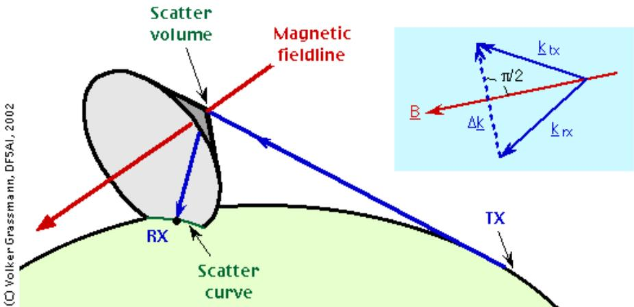
**Figure 1.** The cone of scattering in Aurora and FAI radio propagation.
