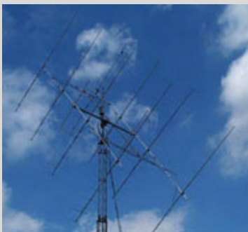
Abb. 1. 144 MHz Antenne, DL1EJA in JO31DS.
