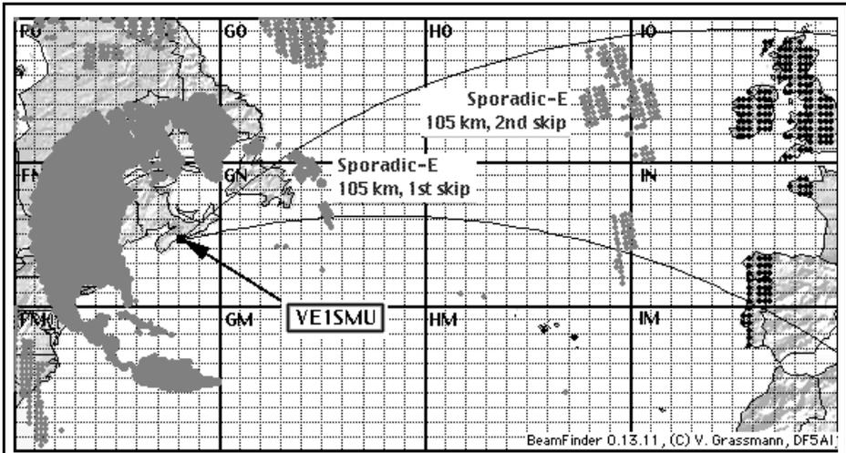
**Fig 4: Possible reception of beacon VE1SMU is Portugal, Spain, France, Ireland and Great Britain (black). The reflections on the ionosphere are to the east and south of Newfoundland (first skip) and on the edges of locator squares HO and IO plus in the east the HN square (second skip).**
